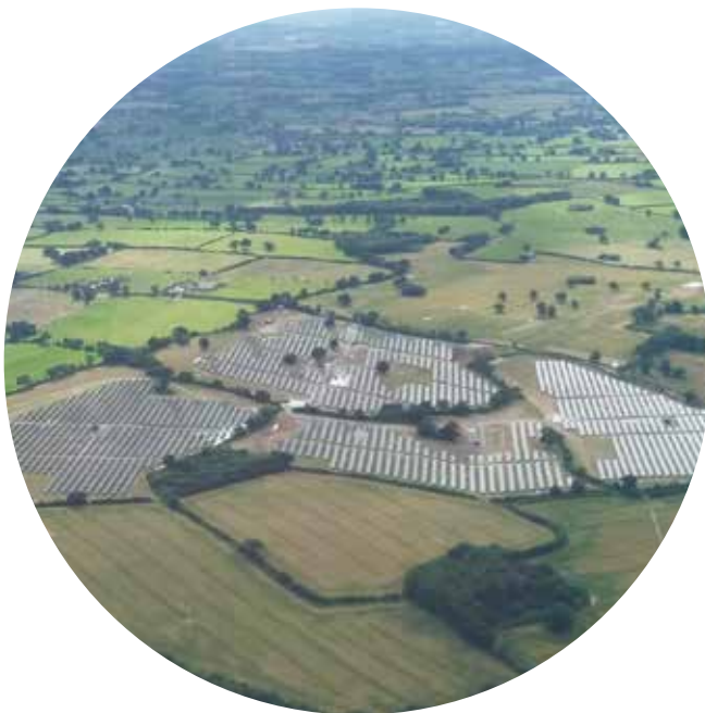
©Lightsource Charity Farm solar project across 86 acres with up to 54,349 solar panels with an installed capacity of 11.9MW.
